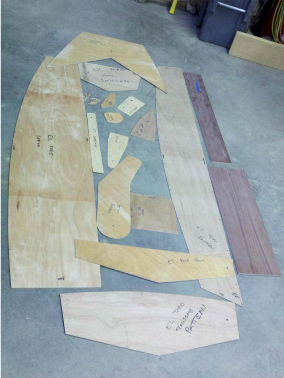
carefully trace around the patterns on 4mm Okoume plywood as per the thickness marked on the patterns.
