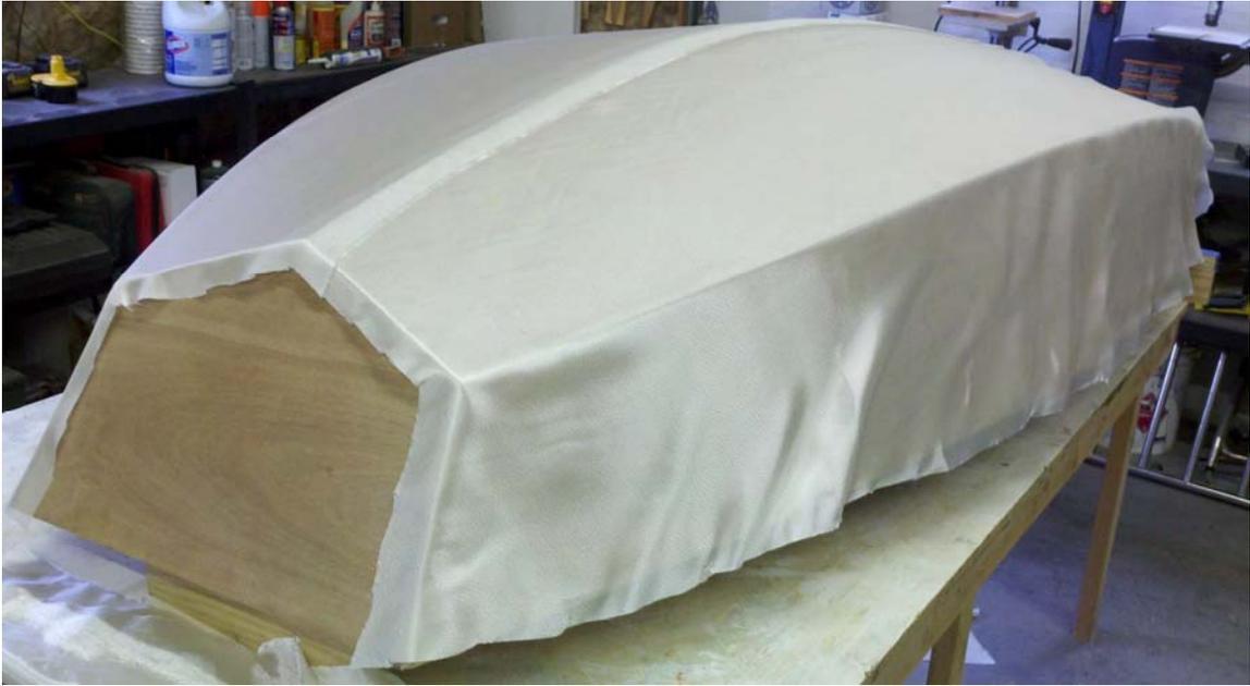
Try to keep the excess resin to a minimum. The cloth should have a satin look when finished. Lightly sand the seams and trim the overhang after the epoxy has cured.
