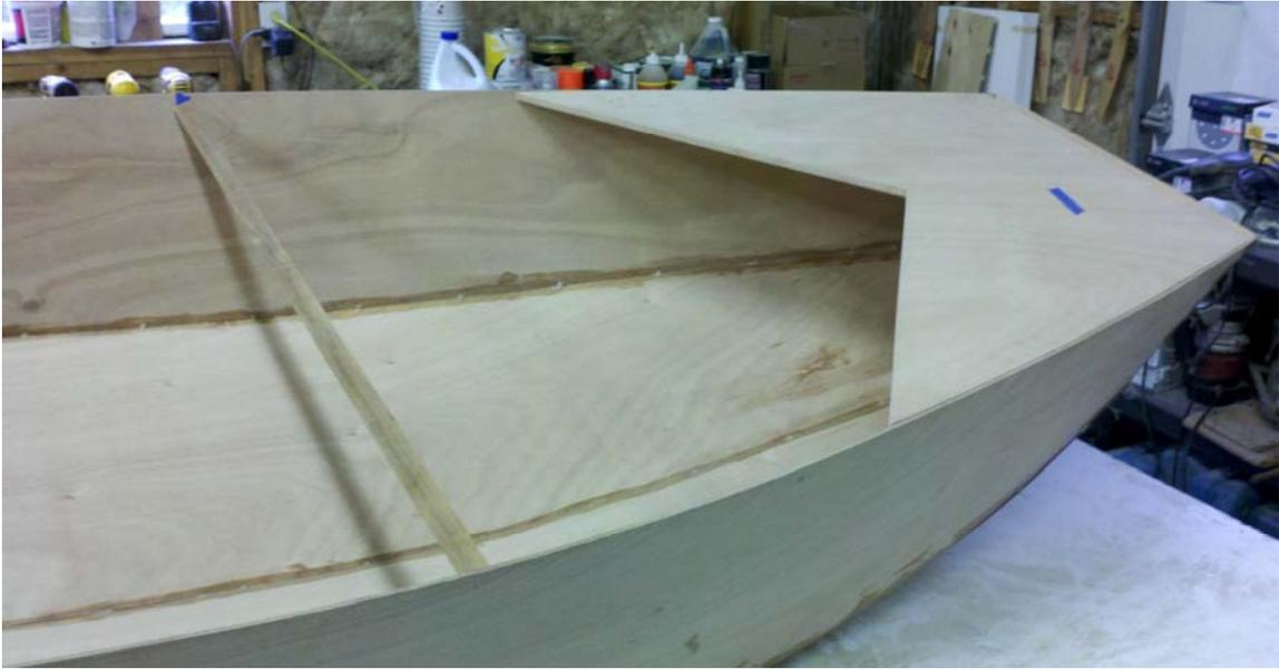
Flip the ET over. Tighten and straighten the seams.
