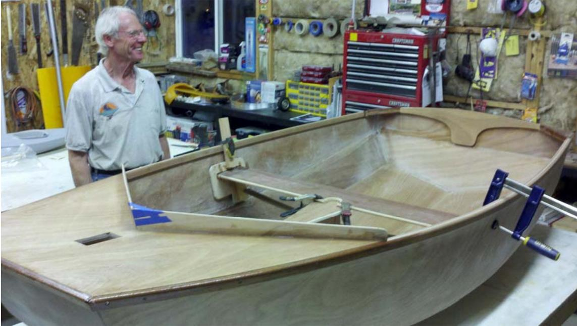
Roll the ET over and roll epoxy over the outside of the hull. After it has hardened, sand the outside with 120 grit sandpaper and start the varnishing process. We recommend a good quality UV rated spar varnish to seal the entire ET. Lightly sand between coats using 220 grit sand paper. The final coat can be sprayed or slowly brushed using foamy brushes.
