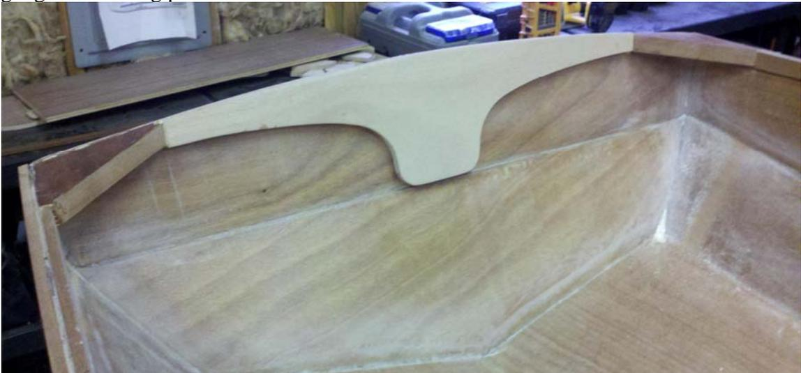
Glue the mast step in place and fiberglass all four sides. Make sure the mast is square to the deck.
