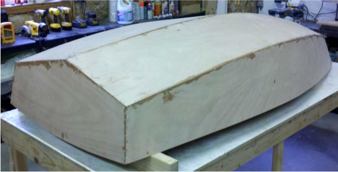
Remove all the stitches and sand the outside of the hull and sand the outside. Roll the ET over and glue the rudder mount backing plate as close to the bottom of the ET as possible. Add a one inch strip of fiberglass tape to all the seams.
