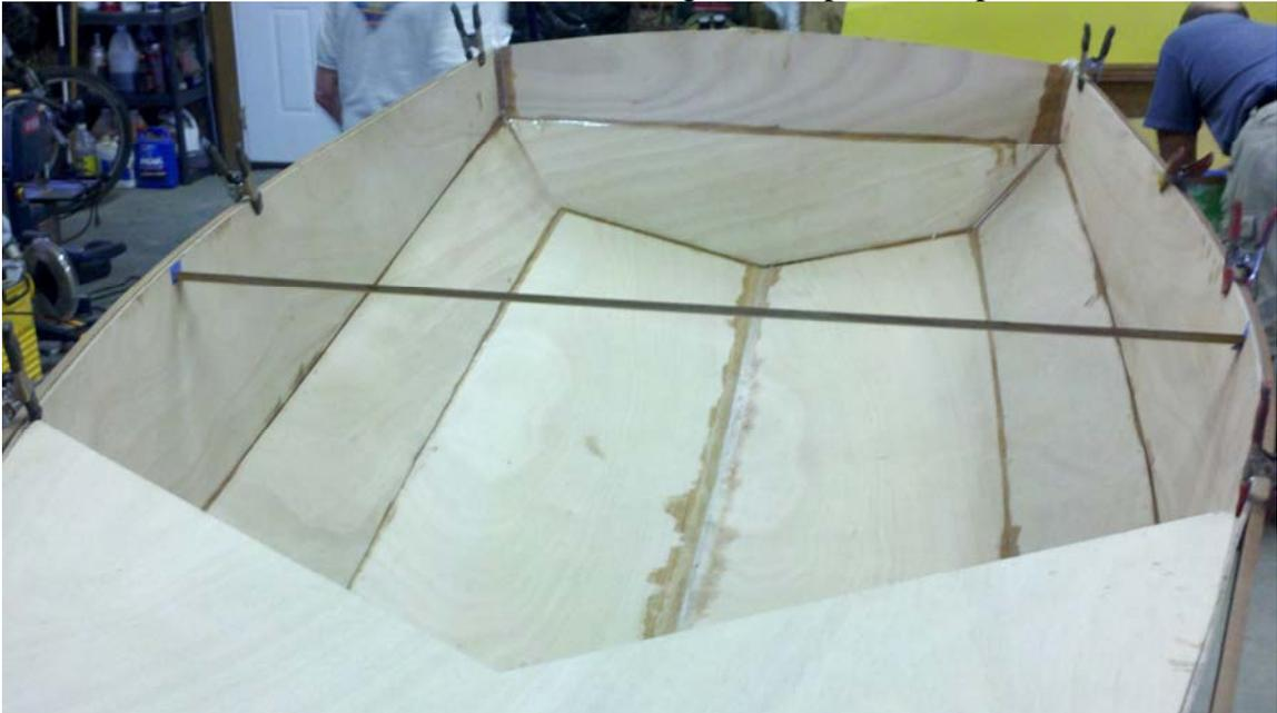
Lay the inside cloth on the hull and carefully smooth by hand. Trim the cloth leaving one extra over the tanks. Add the side and end pieces of cloth after apply the resin in the bottom.
