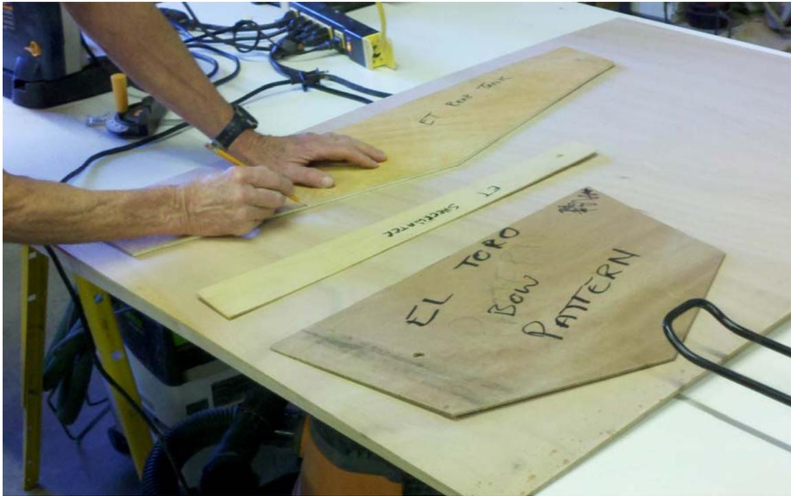
Use a band saw or jigsaw to cut on the outside of the pencil lines. Sand or plane the lines to the pencil lines by hand. Look down the edge and make certain the curves are fair with no flat spots.
