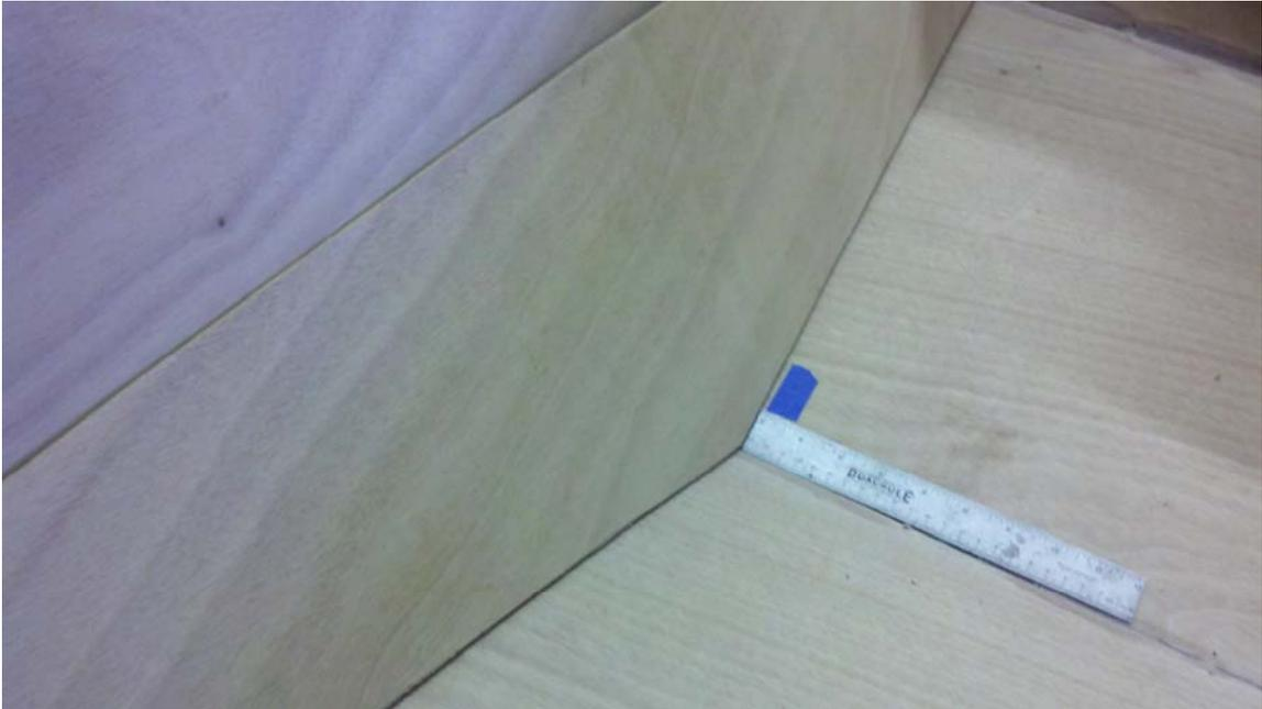
Trim the side flotation tanks and tack nail them into place. Brush thickened epoxy over the seams. Remove the nails, sand the excess epoxy and glass over the inside. You might want to remove the deck at this time. Leave the gunwale spreader in place.
