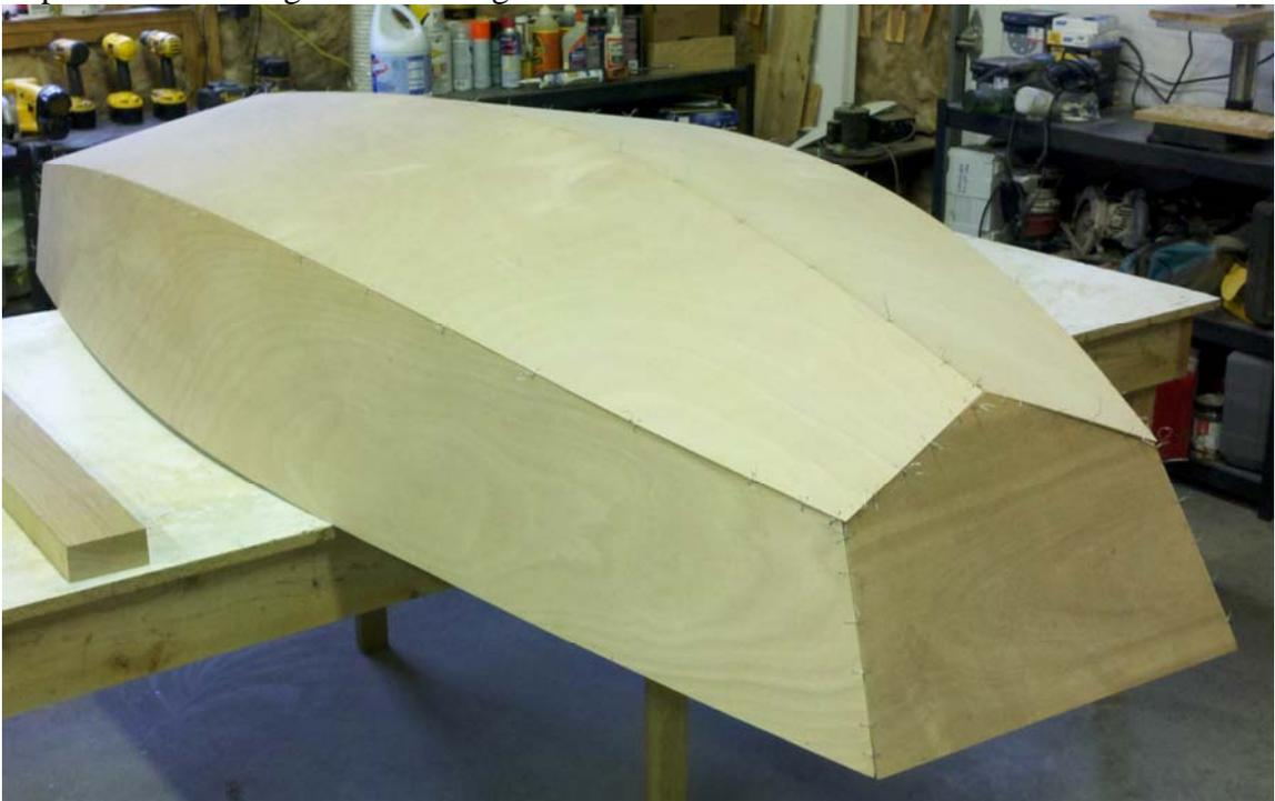
Brush thickened epoxy on all the seams inside and out. Keep the ET flat by letting the bow sit on your bench and use equal height blocks on the transom. Let the ET sit overnight.
