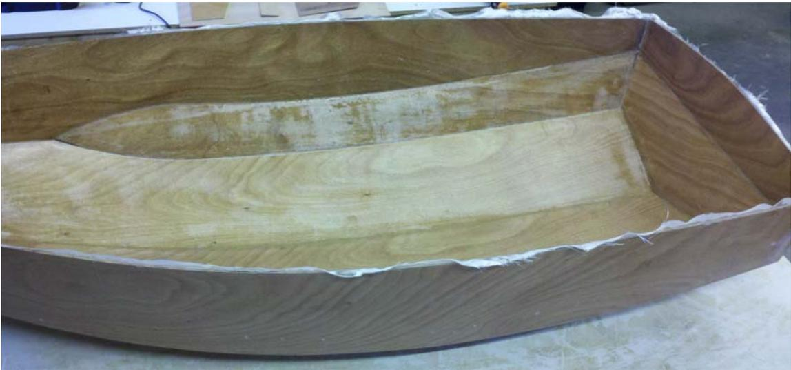
Lay the fiberglass cloth on the hull starting from the keel to the gunwales. Get yourself one inch extra all around. This will get you double overlaps at the keel, bow and stern. After you spread the epoxy add the bow and transom cloth.
