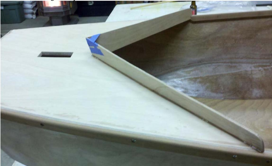
Test fit the seat, seat support and centerboard truck. Use the class rules for placement. Carefully check the truck to be centered in the hull and aligned with the mast/rudder. Take your time! When are you happy with the fit epoxy all the parts at one time and clamp in place. Check the truck alignment. Spread thickened epoxy around the truck base and place fiberglass cloth of the fillet. Rejoice, because you are nearly finished.
